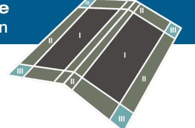
Standard industry wind tunnel tests on various roof configurations have shown that the wind loading on a roof is divided into three zones:
