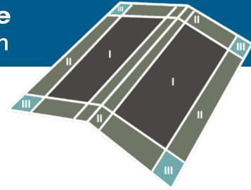
Standard industry wind tunnel tests on various roof configurations have shown that the wind loading on a roof is divided into three zones:
